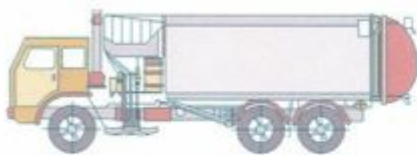
Side loading collection vehicle for MGBs (Mainly used for domestic waste collection)
