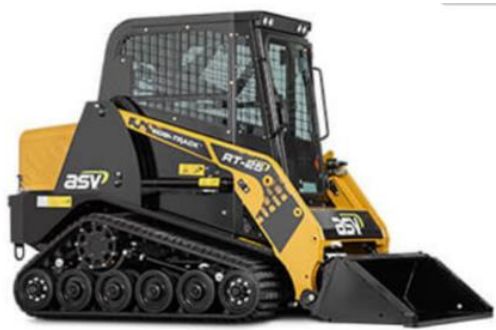
Figure 1: Pos-track – used for loading substrate onto the barge
