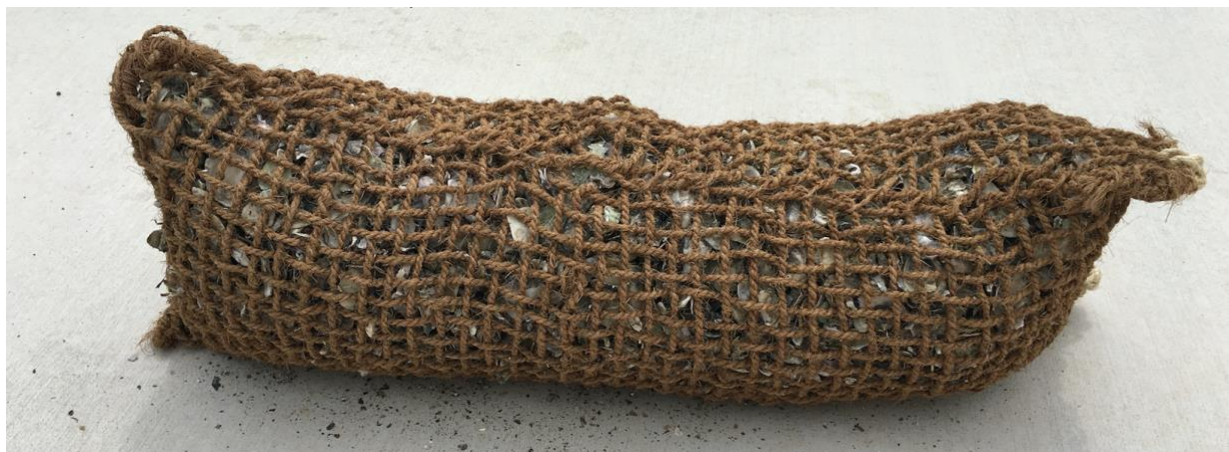
Figure 1 Coir mesh bag filled with recycled oyster shells; the principle restoration unit
